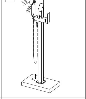
5. Tighten screws(3) with allen key(11). Then connect hand 6. Check for leakage after installation. Finally, push down shower(8) and Main body with shower hose(9).
