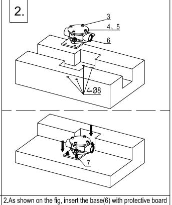
After selecting proper position, drill a mounting hole as shown above. If the thickness of decoration layer ≥ 50mm, please install on the floor directly. 2.As shown on the fig, insert the base(6) with protective board (4), washer(5) and expansion plug(7) to mounting hole. After adjusting proper position, mark the drill holes accordingly. Then drill 4 holes with size Ø8 on the marking places, then put the expansion plugs(7) into the holes respectively.
