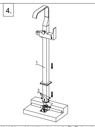
furnish the floor according to the construction. Remove the 4.Install the mainbody(1) as shown on the Fig. Fix the main protective ring, screw(3), protective board(4) and washer(5) body on the base with screws.
